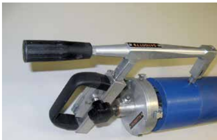
2. Use scraper to remove oxide layer approx. 0.3mm from pipe and ensure correct tolerance.
