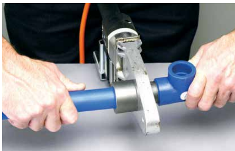
3. Simultaneously insert pipe and fitting onto socket and spigot to full depth without twisting. Hold for 'pre-heat' time as per table.
