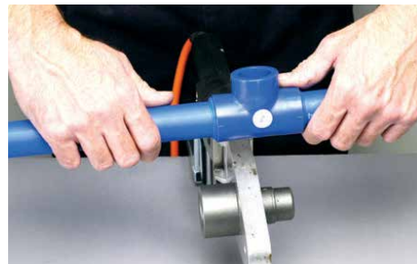
5. Check alignment within 'adjusting seconds' as per table. During 'cooling' avoid mechanical strain or movement on welded joint.
