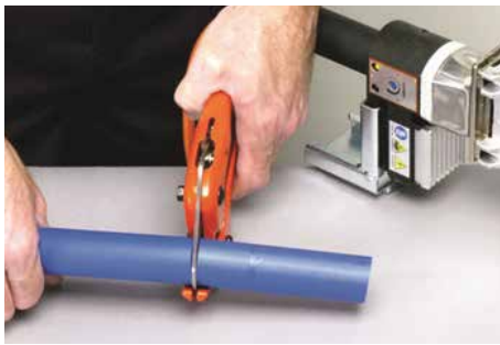
1. Turn on welder. Do not attempt welding unless tool is up to temperature (250°C). The indicator LED will cycle on/off with thermostat control when temp is correct. Cut pipe to length with approved cutters for a square swarf-free finish.
