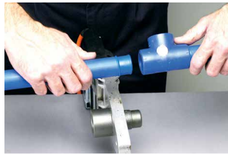
4. Remove pipe and fitting from heating element, immediately insert pipe into fitting without twisting.
