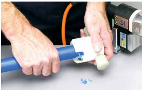
2. Use scraper to remove oxide layer from pipe and ensure correct tolerance. Use welding wipes to clean surfaces if needed.
