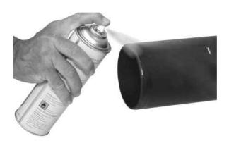
4. Apply silicone oil on rubber seal and sparsely on spigot end.
