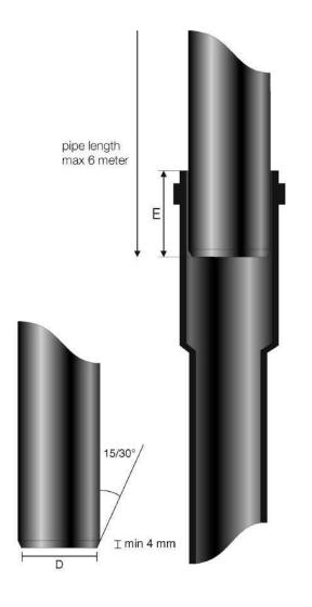
Expansion joints are push-fit sockets with a rubber seal.
