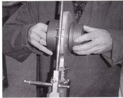
Fig. 2 Place the socket and the spigot on the heat reflector
