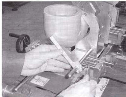
Fig. 7 Adjust the stop to hold the fittings
