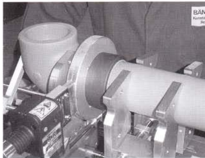
Fig. 9 Move the machine slides with the handle lock, warmup the pipe and the fitting in the welding tools
