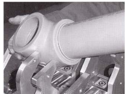
Fig. 12 Remove the welding jointing after the cooling time from the clamping jaws has past
