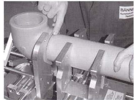
Fig. 8 Lay the pipe axial to the fitting and position it so that is situated frontal to the fitting
