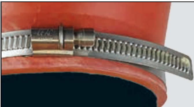
CaseCore Compenseal steel strap width 20 mm for pipe size OD 75 mm up to 280 mm, Torque value 10 N
