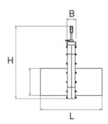
Note: 110/125mm are SDR17 pipe tails. 160-315mm are SDR26 pipe tails. Other SDR pipe ends available on request. 3-4 week lead time may apply.
